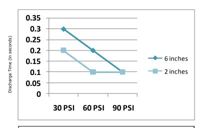
Offset voltage and discharge time per ANSI/ESD STM3.1 using a charged plate monitor with a 20pF, 6" x 6" plate. 1000 to 100 volts. Typical results.
