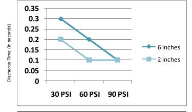
Offset voltage and discharge time per ANSI/ESD STM3.1 using a charged plate monitor with a 20pF,  $6^{\prime\prime}$  x  $6^{\prime\prime}$  plate. Typical results. 1000 to 100 volts.
