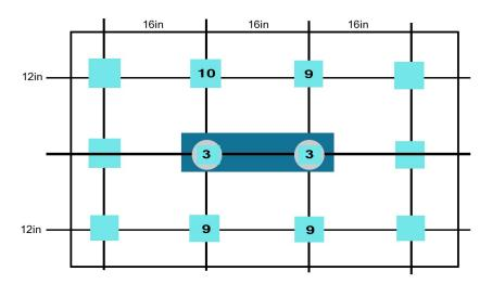
Offset voltage and discharge time determined using charged plate monitor. Discharge times are in seconds from 1000V to 100 V
