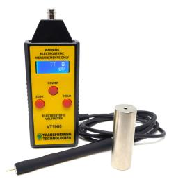
hand-held probe is included in its standard configuration, which can be used to test human walking voltage.
