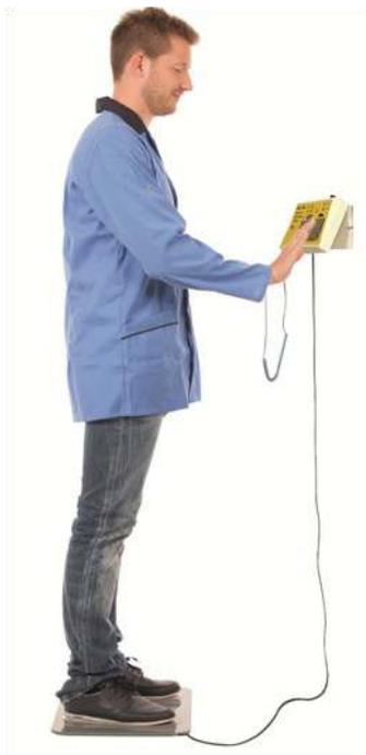
The PGT120 is supplied complete with footwear testing electrode, flexible cord, transformer with power cord and calibration protocol. Recommended calibration interval is 24 month. Corresponding wall mounting plate, and electrode anti-fatigue mat is sold separately.
