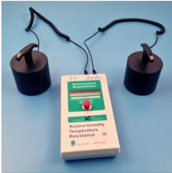
Figure 3 – Resistance Point To Point (RTT)
