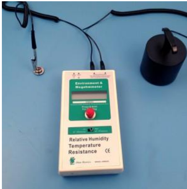
Figure 2 – Resistance Point To Groundable Point (RTGP)
