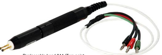
Replaceable head 844 (Two-pointprobe) with conductive rubber tips, for <u>rigid</u> materials testing.
