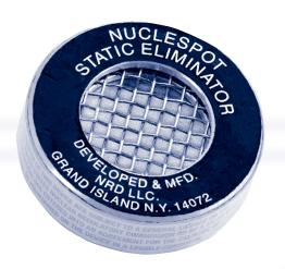
The model **P-2042** Nuclespot Alpha Ionizer is a small, self powered ionization device that quickly eliminates static charge. It's designed for use in a variety of applications where space is limited, and is ideal for installation inside equipment. Test results have shown that alpha energy ionizers are the only technology that does not contribute to increased particle levels in the environment.
