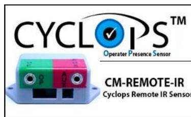
CYCLOPS™ protects ESD safe workstations by sensing when an operator is within the protected work area and alarms if a wrist strap is not connected. The alarm continues until compliance is achieved, preventing isolated operators from damaging ESD sensitive devices.
