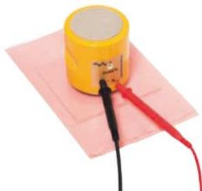
Sample application: measurement with concentric ring probe
