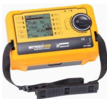
7100.3000.G * High resistance meter with connecting cables
